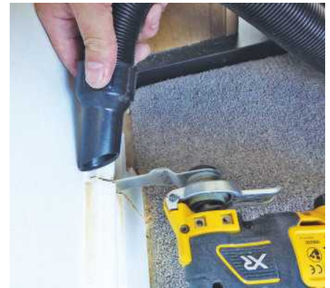
▶ The vac is ideal for capturing localised dust when working in situ
